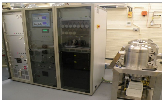
FIGURE 22. The UK CTBT radionuclide noble gas laboratory (GBL15), which uses a SAUNA II IMS lab system to process and measure radon samples from the IMS noble gas station network.
