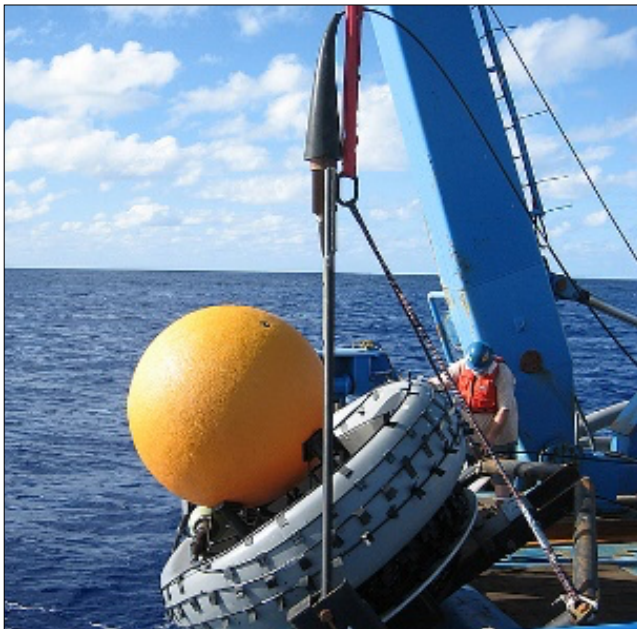
FIGURE 12. Deployment of a hydroacoustic node from the aft deck of a ship. The large yellow sphere is the mid-water float. The riser cable can be seen wrapped around the circular anchor.
