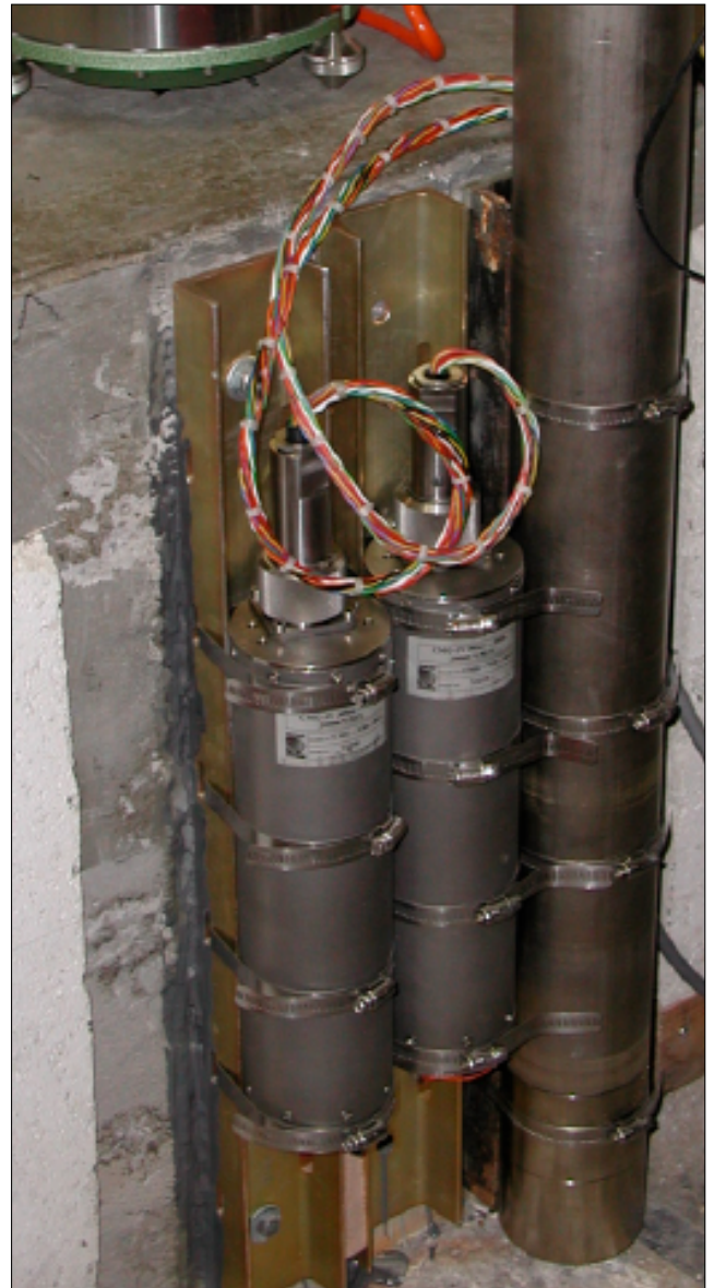
FIGURE 10. Testing of the borehole version of CMG 3 type of instruments clamped to the concrete wall with special fixtures (courtesy of SNL testing reports, for example: Hart and Merchant 2014).
