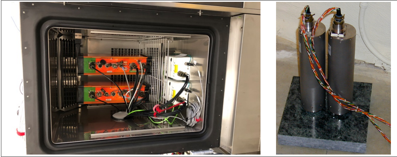
FIGURE 11. Self-noise testing of Q330M+ (Kinemetrics, USA) and Centaur (Nanometrics, Canada) digitizers inside the temperature chamber at SNL (left panel) and side-by-side testing of two CMG3V vault seismometers at the right panel (courtesy of SNL testing reports).
